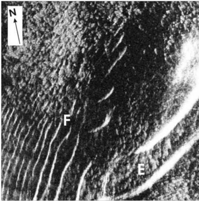
Figure 7. Extract at full resolution of an Envisat ASAR image (WS mode) from 20 February 2006 (yellow waves in Figure 1) showing two distinct wave packets (E and F). The image size is 38 km \times 38 km and its center is at (20.72°S, 36.48°E).
